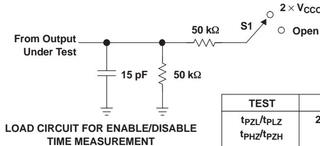
LOAD CIRCUIT FOR ENABLE/DISABLE TIME MEASUREMENT
